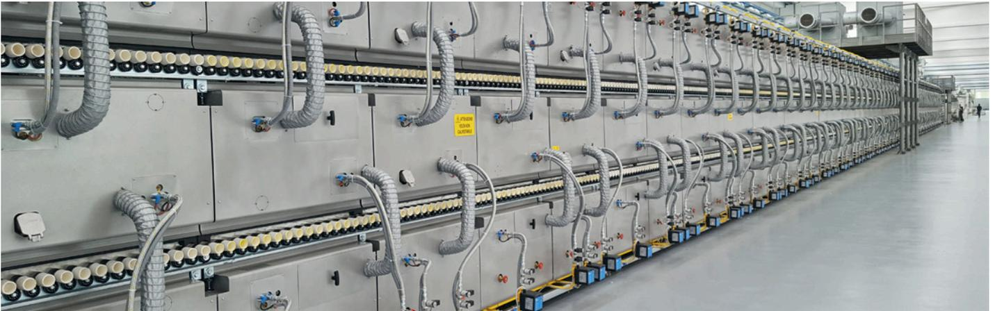
The growing production of large size tiles in the ceramic sector has given rise to a new problem: the elimination of residual post-firing stresses to allow for subsequent operations of cutting, drilling, etc. For this purpose, large size tiles need to be fired for much longer times than medium-sized tiles, regardless of the stresses generated in the previous steps.
